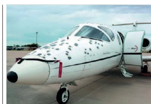
That's a T-1A Jayhawk blemished from a hailstorm that swept through the Laughlin Air Force Base in Texas in 2017. That damage is severe enough to require skin replacement.
